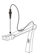
Insert the connector of temperature probe into corresponding connector socket (Marked "ATC").
