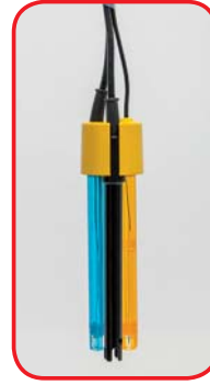
Electrode holder for field application with 3 holes
