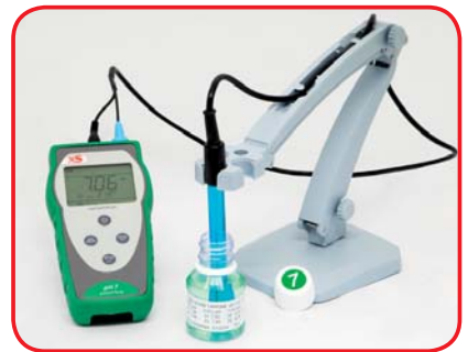
Electrode holder for use on laboratory bench (optional)
