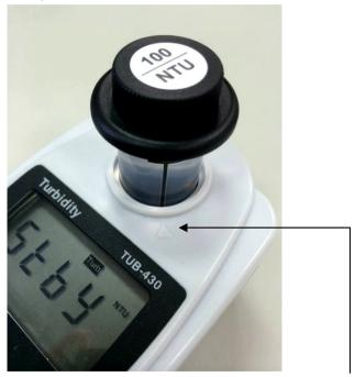
During calibration or measurement, please make the line on the bottle aligned with the arrow on the meter.
