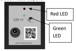
If both lights are on and there is no ERROR message on the screen, the unit will be at temperature and only small, fast pulses of heat are required. In this condition, the lights will be switching on and off very fast and may give the impression that they are on all the time.
